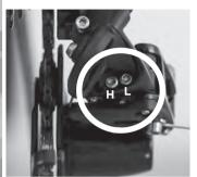
The limit screws prevent your chain from exceeding the limits of the cassette. You have one screw controlling the higher limit (H) and one screw for the lower limit (L). The higher limit corresponds to the smallest cassette ring while the lower limit corresponds to the biggest cassette ring.
