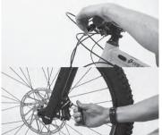
Whilst holding the brake lever, tighten the caliper bolts.
