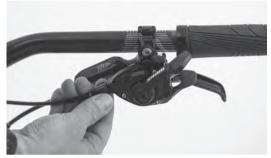
Once your limit screws are set, you have to adjust the cable tensionner. Try shifting through the gears:
