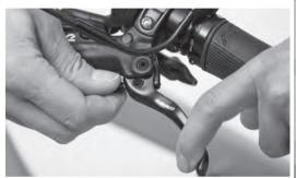
You can adjust the reach of the brake lever. Simply turn the fine adjuster found on the brake lever. This can also be in the form of an allen key bolt.
