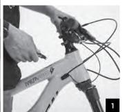
If prefered, you can adjust your handlebar height by modifying the spacer stack. To do so, unscrew and remove the topcap. Then, untighten the stem bolts. Remove the stem and adjust the spacer stack to change height.
