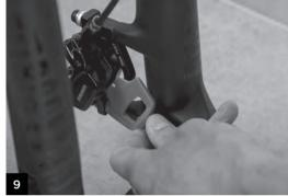
STEP 9 Remove the pad spacer from the caliper, Keep the spacer to aid in transportation in the future.
