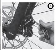
To align the caliper to the disc, unscrew the two bolts by half a turn so it is fairly loose. Turn the wheel and press the corresponding brake lever.
